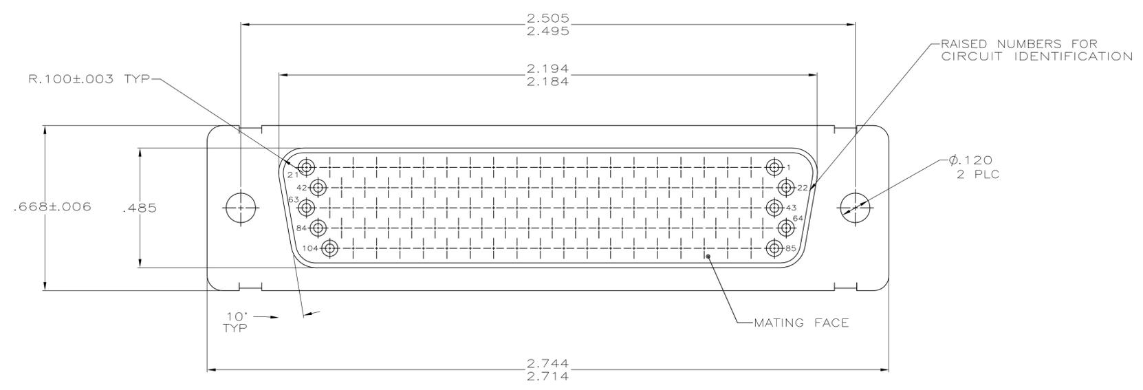
1. THIS RCPT. WILL MATE WITH ANY SIZE 6, 104 POSN. PLUG IN AMPLIMITE SERIES.
