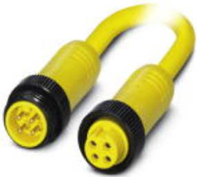
Power cable, 4-position, PVC, yellow, Plug straight 7/8"-16UNF, on Socket straight 7/8"-16UNF, cable length: 10 m
