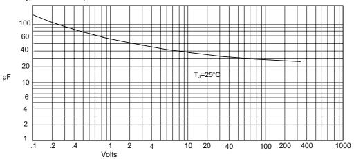
Junction Capacitance - pF*versus* Reverse Voltage - Volts
